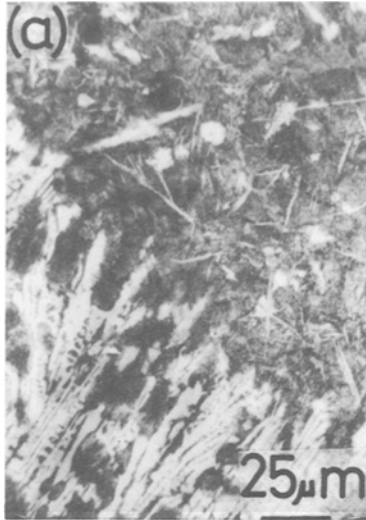
Figure 6 Microstructure of the fusion boundary and the HAZ of FGI deposited with iron filler metal by a plasma arc using argon plasma gas and Ar + 10% H 2 shielding gas at an arc current of 130 A. Nital etch. (a) Deposit fusion boundary region. (b) Fusion boundary region having ledeburite adjacent to pearlite on the iron deposit metal side. (c) Columnar structure consisting of ferrite and pearlite on the deposit metal side of the fusion boundary. (d) Ledeburitic layer in the HAZ. (e) Eutectic graphite layer appearing in the HAZ.
